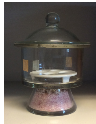
Figure 2.11 Example of a desiccator. The solid in the bottom of the desiccator is the desiccant, which in this case is silica gel.
