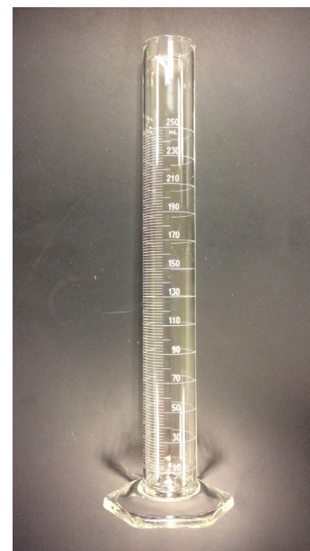
Figure 2.4 An example of a 250-mL graduated cylinder.
