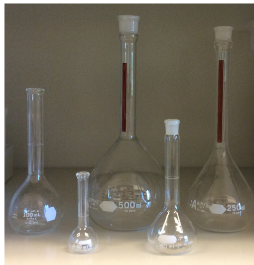
Figure 2.7 A collection of volumetric flasks with volumes of 10 mL, 50 mL, 100 mL, 250 mL, and 500 mL.
