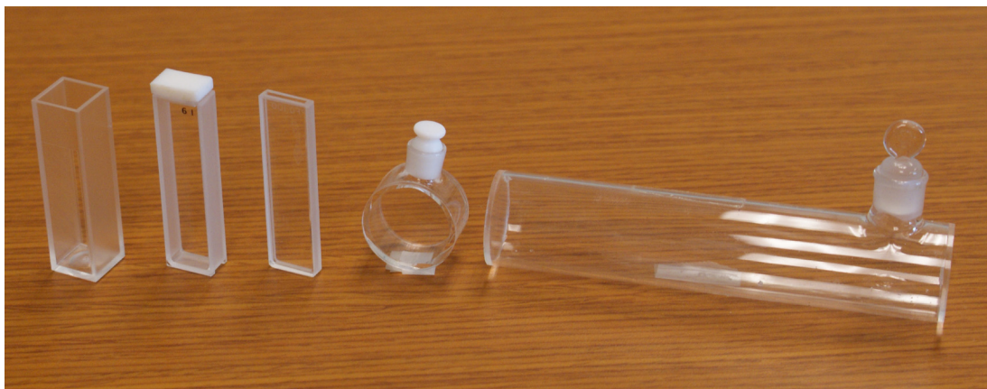
Figure 10.30 Examples of sample cells for UV/Vis spectroscopy. From left to right (with path lengths in parentheses): rectangular plastic cuvette (10.0 mm), rectangular quartz cuvette (5.000 mm), rectangular quartz cuvette (1.000 mm), cylindrical quartz cuvette (10.00 mm), cylindrical quartz cuvette (100.0 mm). Cells often are available as a matched pair, which is important when using a double-beam instrument.
