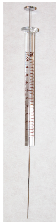
Figure 12.29 Example of a syringe for injecting samples into a gas chromatograph. This syringe has a maximum capacity of 10 µL with graduations every 0.1 µL.
